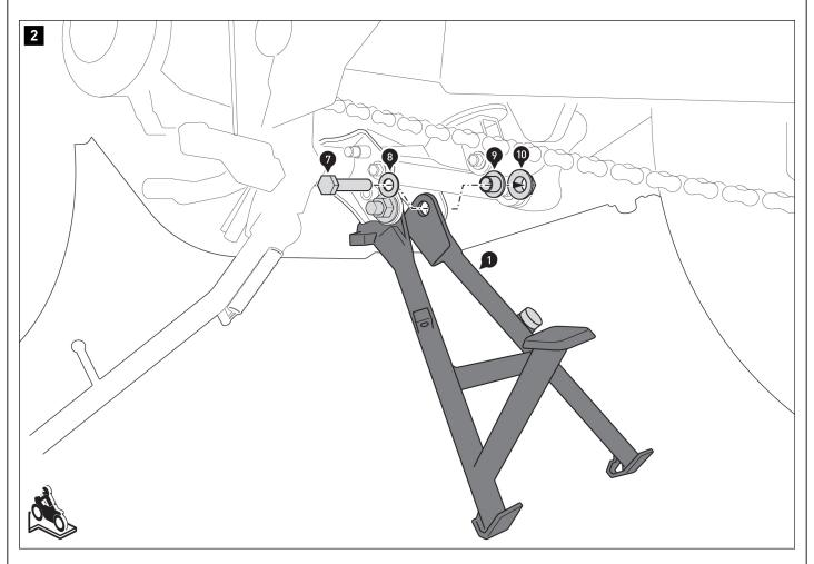
Coat the outside of the bearing bushing (9) with grease.
