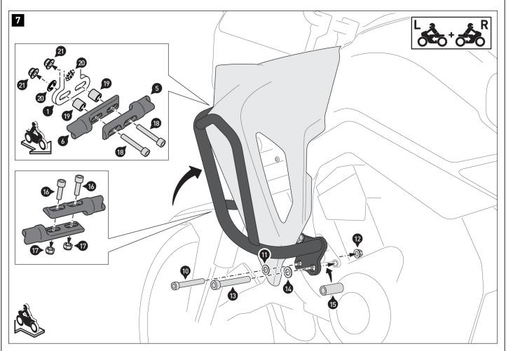
Screw the crash bar halves (5) and (6) to the two remaining attachment points
