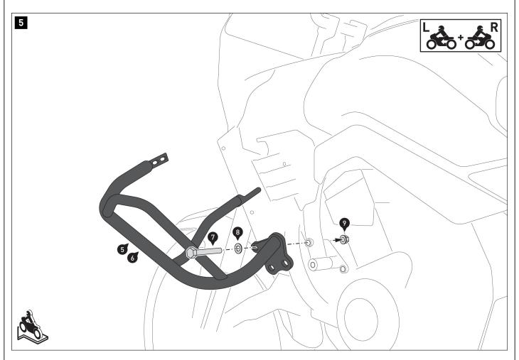
▲ WARNING: Cover the fender to protect it from any accidental scratching!
