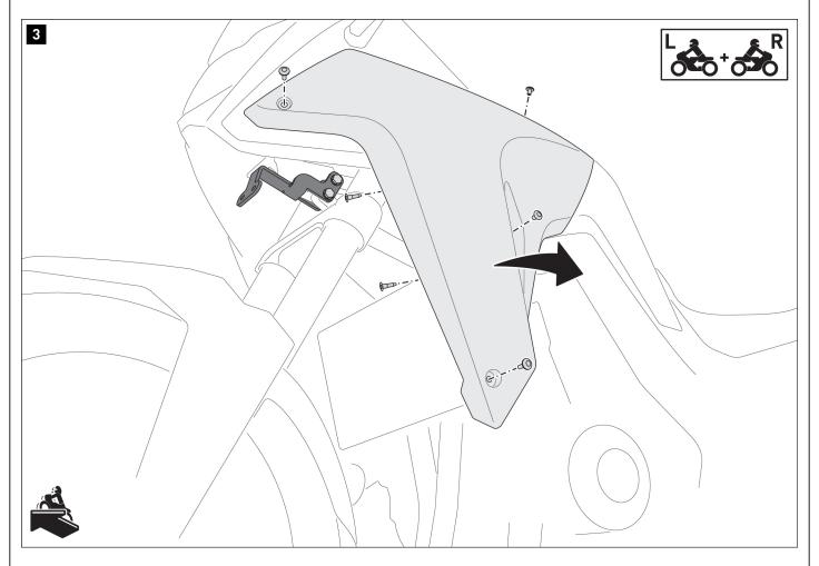
f A NOTE: The following steps indicate how to mount the left crash bar (5). Assemble the right crash car (6) in the same way.
