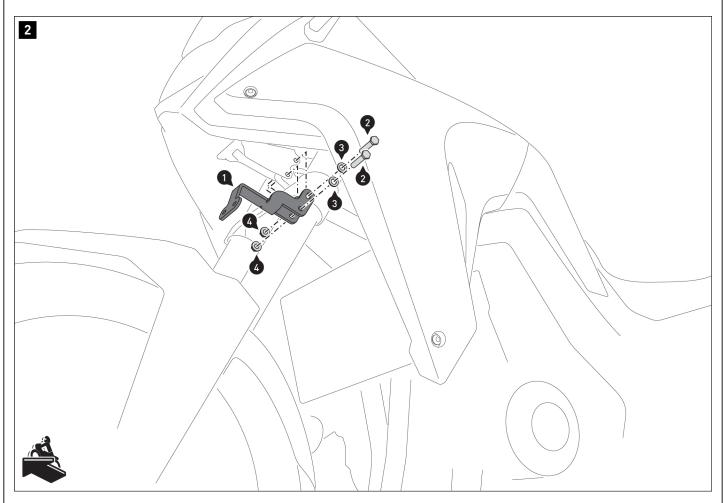
Screw on the mounting bracket (1). Tighten the screws as specified.
