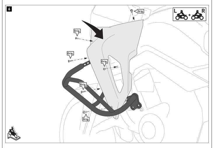
$\begin{tabular}{ll} \bf OPTION~[1]: Mount~the~side~panel~in~this~step.~Tighten~the~original~screws~ (Orig.)~according~to~the~manufacturer's~instructions. \end{tabular}$
