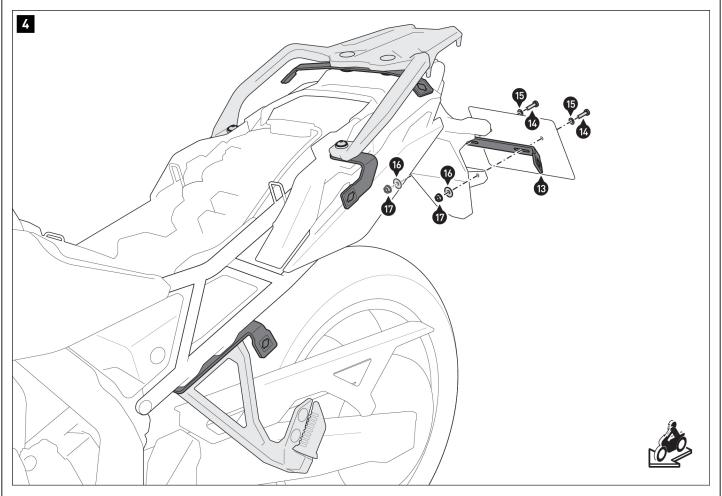
Screw the crossbar (13) together with the license plate to the license plate holder. Do not tighten the screws yet.
