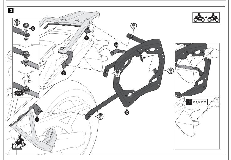
Connect the side carriers (10) and (11) to the fastening straps (1), (2), (5) and (6) and crossbars (7) and (13) using the quick-release fasteners (12). Secure the quick-release fasteners using the lock washers.
