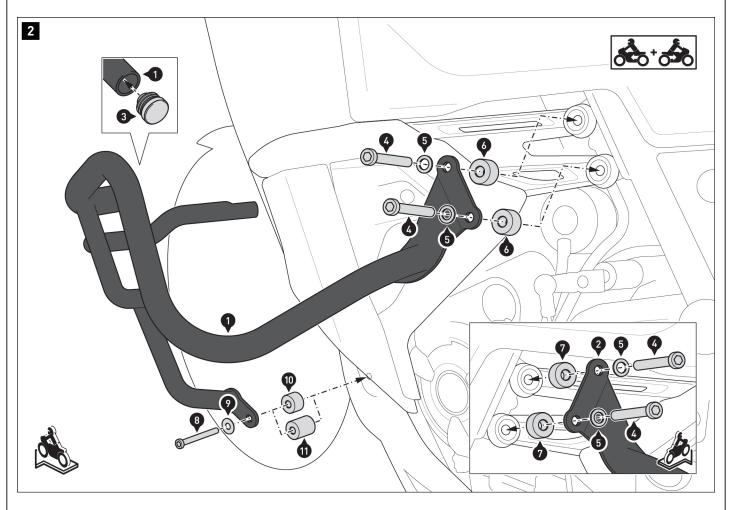
Screw the left crash bar (1) to the vehicle. Note that spacers of different heights are fitted at the rear attachment points on each side.
