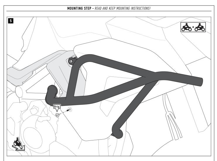
Reattach the side fairings to the vehicle. Tighten the original screw (Orig.) according to the manufacturer's instructions.
