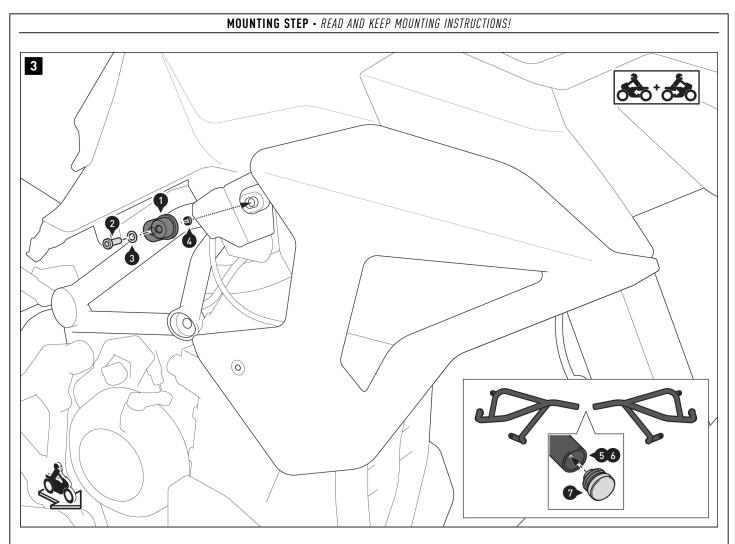
Screw the mounting bracket (1) under the rubber trim to the vehicle. **A WARNING: Use a liquid threadlocker!** Do not tighten the screw yet.
