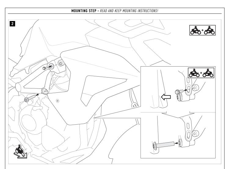
Remove the screws indicated from the vehicle.
