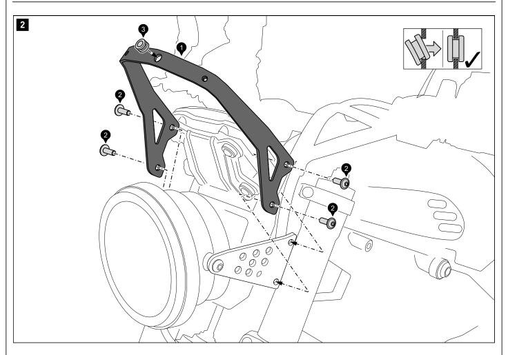
Insert the rubber grommet (3) into the mounting bracket (1).
