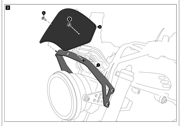
Screw the windscreen [4] to the mounting bracket [1]. **A WARNING: Use liquid threadlocker!** Tighten the screws as specified.
