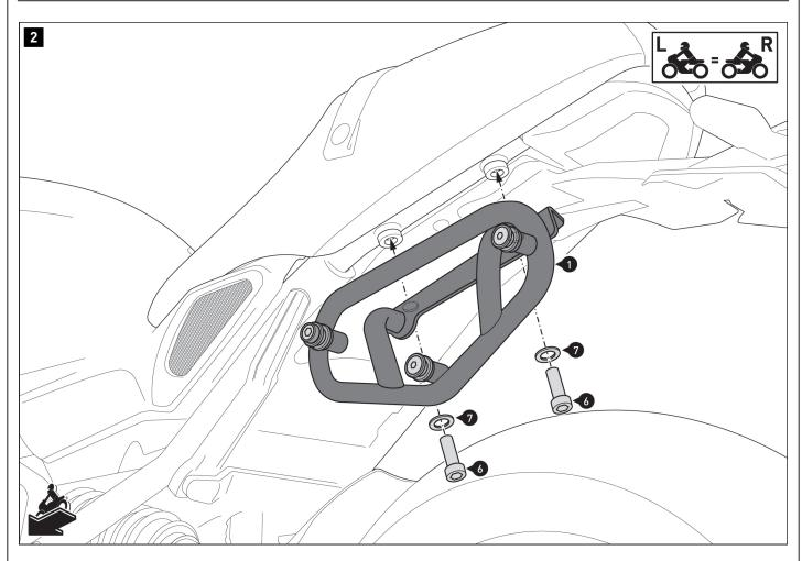
Screw the side carrier [1] to the rear of the vehicle. **AWARNING:** Use a liquid threadlocker! Tighten the screws as specified.
