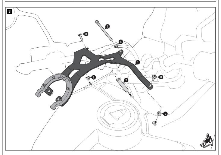
Screw the mounting bracket (1) to the vehicle. **A** WARNING: Use a liquid threadlocker!
