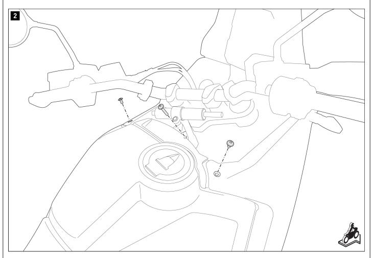
Remove the original screws from the attachment points shown.
