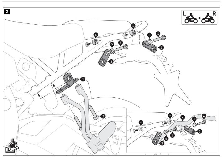
Screw the mounting brackets (1) to the passenger footrests on both sides of the vehicle. **AWARNING: Use a liquid threadlocker!** Do not tighten the screws (2) yet.
