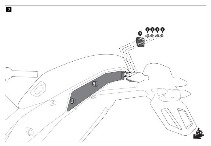
Connect the cover plates [1] and [2] to the connecting plate [5].
