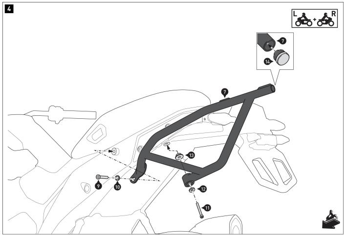
Insert the plastic plugs (14) into the ends of the mounting struts (7/8).
