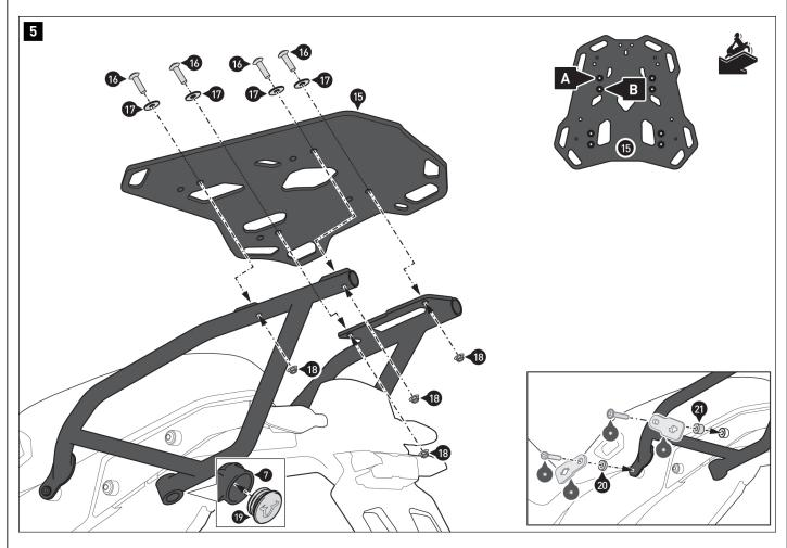
⚠ **NOTE:** If the SW-MOTECH side carrier is installed at the same time, screws (3) and (9) are omitted. In their place, mount the screws (\*) included with the side carrier as shown in the detailed drawing below.
