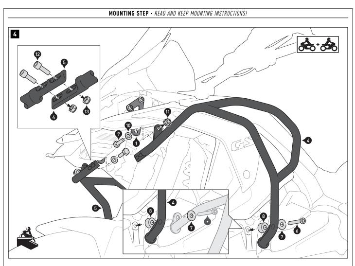
$\triangle$  **NOTE:** If this product is to be installed with the SW-MOTECH crash bar, the installation situation at the lower attachment point changes (see detailed drawing below). Use the screws (\*) included with the crash bar.
