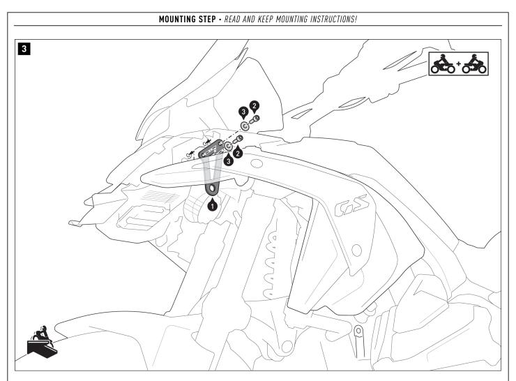
Screw the mounting brackets (1) onto both sides of the vehicle. Make sure to route the cables located at the mounting points past the mounting brackets on the inside.
