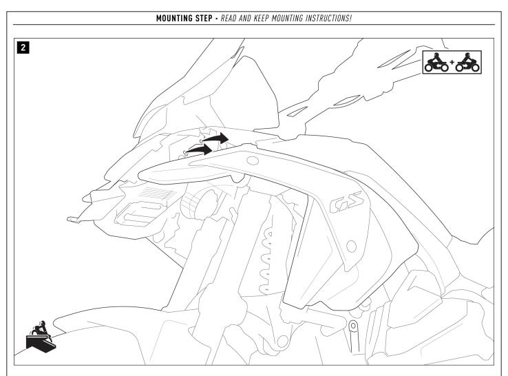
Remove the indicated screws from the vehicle on both sides.
