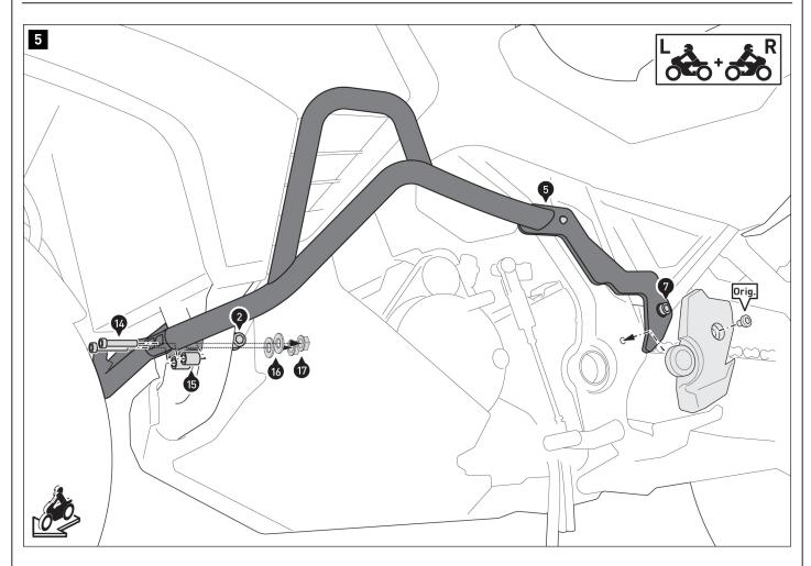
Screw the two crash bars (5) and (6) to the mounting bracket (1).
