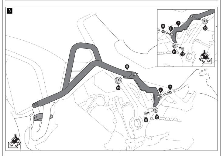
Insert the rubber dampers (13) into the crash bars.
