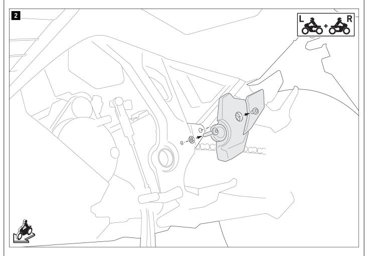
Remove the screws shown and the heel guards from both sides of the vehicle.
