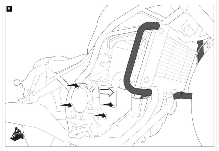
Screw the clutch cover back onto the vehicle. Tighten the screws according to the vehicle manufacturer's specifications.
