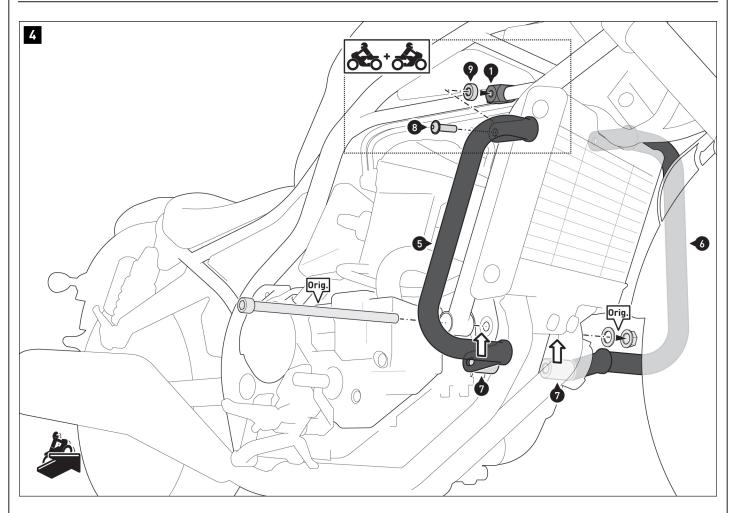
▲ DANGER: For the *Honda CMX 1100 T Rebel* and the *CMX 1100 SE Rebel*, the indicators are attached to the fork bridge! Make ABSOLUTELY sure that the indicators do NOT make contact with the crash bars (5/6) when the steering lock is fully turned! The full steering lock MUST always be maintained! If contact occurs, adjust the frame clamps (1) and crash bars (5/6)!
