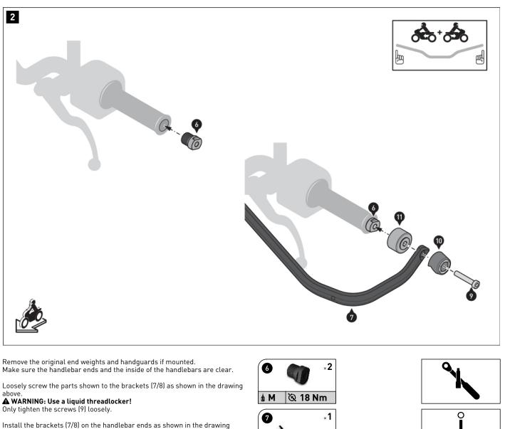
below. To do this, tighten the screw (9) enough so that the brackets (7/8) can still be readjusted.
