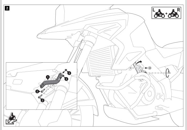
Screw the fully threaded screws (2) into the fork bridge.
