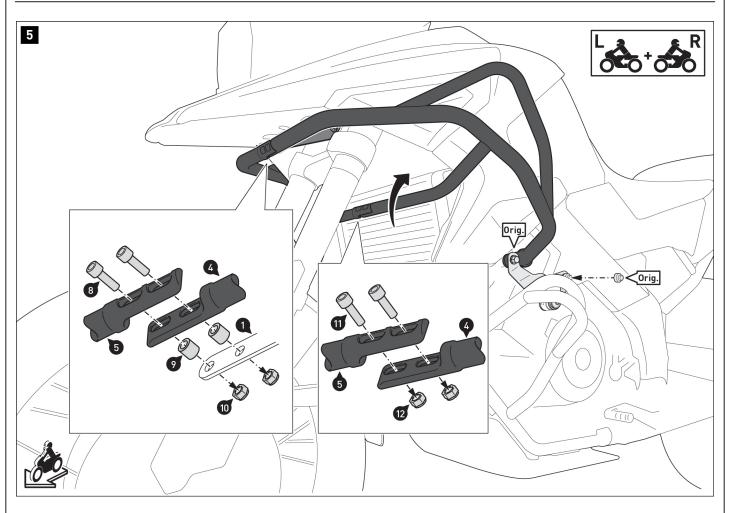
Screw both halves of the crash bar (4) and (5) to the mounting bracket (1).
